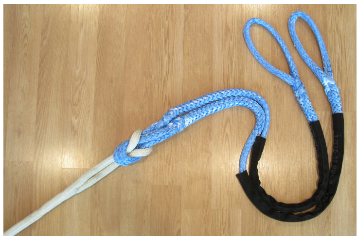
An example of a similar setup used in Nantucket. The bottom white section is made of Nylon and the upper blue section is made from STS-12 SK-75.
