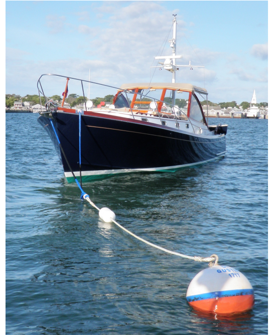
An example of a similar setup used in Nantucket. The bottom white section is made of Nylon and the upper blue section is made from STS-12 SK-75.
